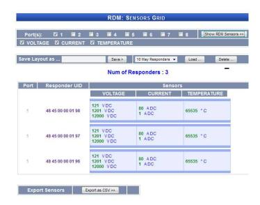
RDM Sensors page, allows discovering all RDM devices and monitoring all sensors supported by RDM tool. Examples include: Temperature, Current and, Voltage sensors.
