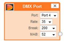
The DMX port represents one of the physical ports on the rear of this unit, select which port you want to use by using the drop down.
