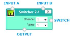
Switcher 2-1: Controllable Switch operator, acts as a normal Input A to Output Action, but when the trigger
